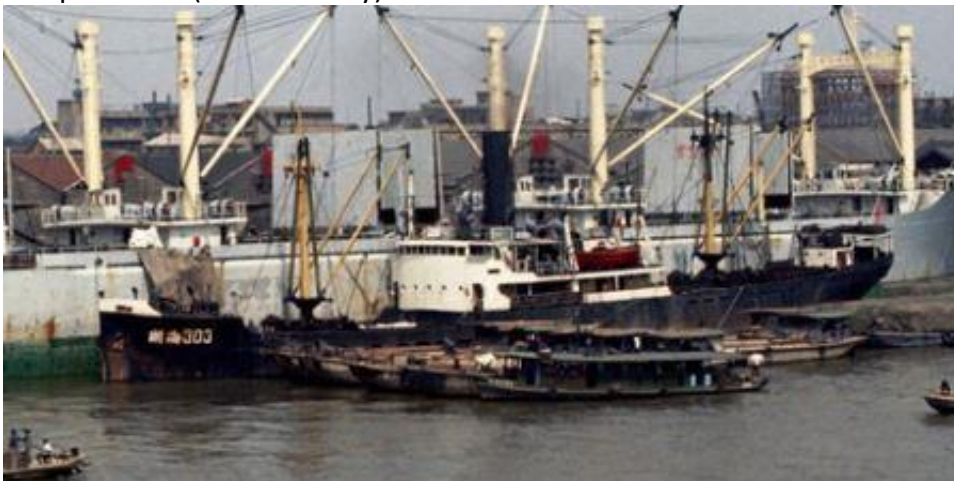
ZHE HAI 303 arriving Shanghai on 18 June 1982 with new masts, superstructure plating, hull openings and portholes (Chris Mackey).
