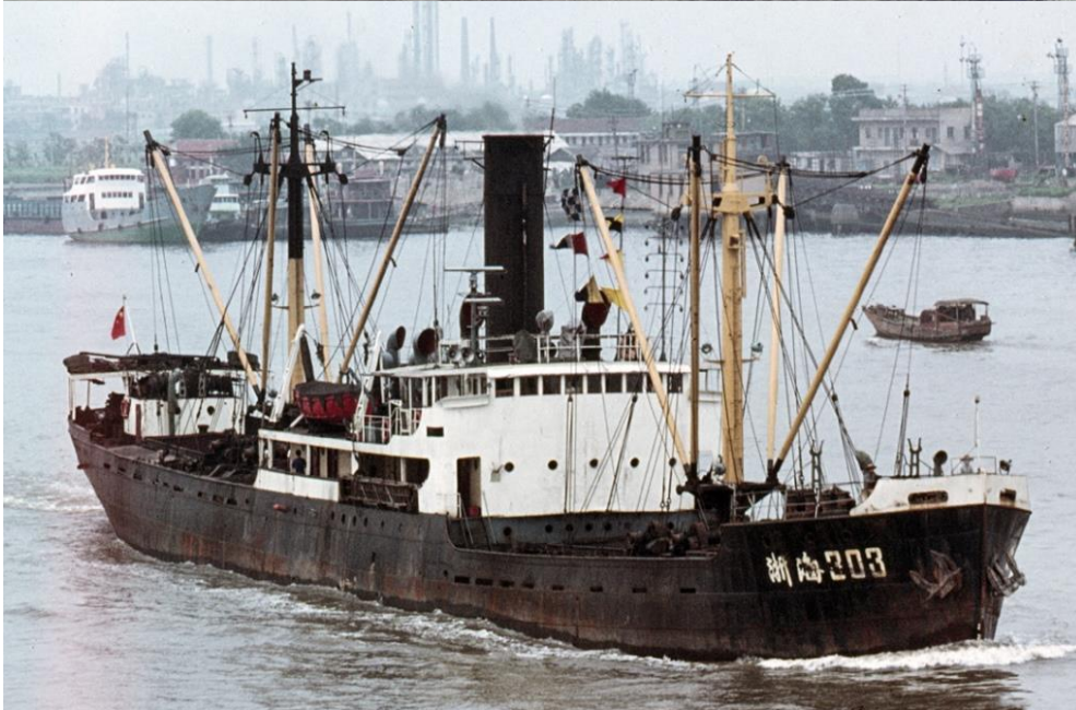
ZHE HAI 303 arriving Shanghai on 18 June 1982 with new masts, superstructure plating, hull openings and portholes (Chris Mackey).
