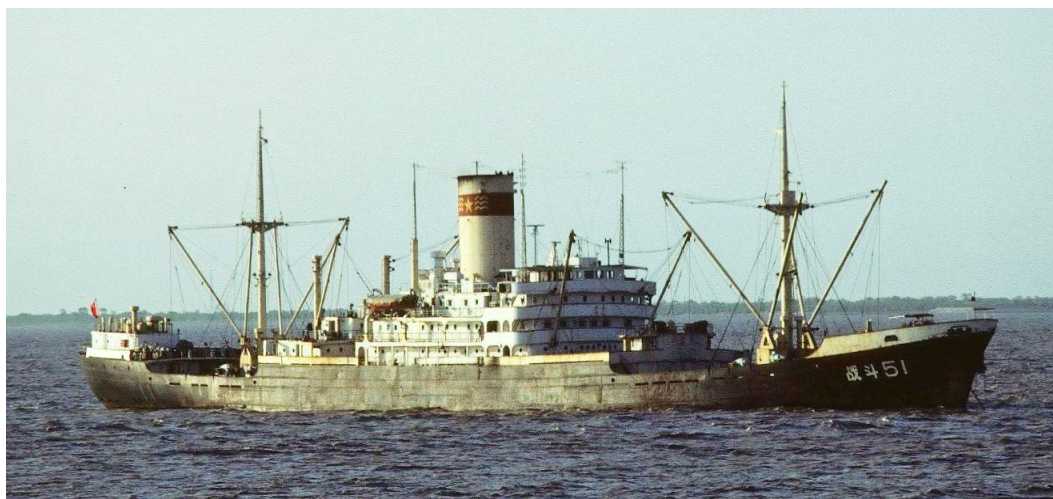
ZHANDOU 51 ex HUNGMIEN in Yangtse delta, three pairs of kingposts removed (Donald Anderson).
