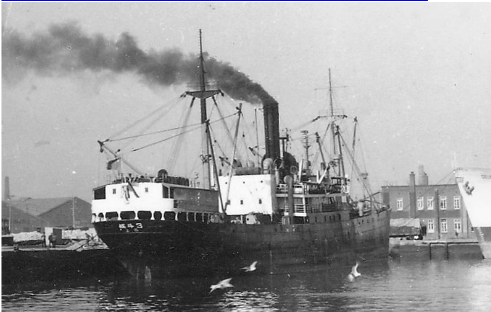
ZHANDOU 3 at Dalian early 1970s. Additional accommodation fitted aft (SK*).
